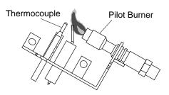
Figure 32 - Incorrect Pilot Flame Pattern (Actual Pilot May Vary From Illustration)
